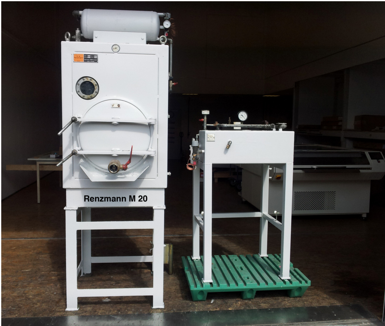
Distillery (Solvent recovery) Renzmann M 20 with vacuum
